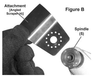
Place the attachment over the Spindle (5), shoulder facing away from the tool. Line up the holes on the attachment with the pins on the Spindle shoulder.
